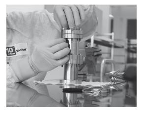
We assemble components and groups of components with high demands on low particle emission under cleanroom conditions. Therefore, cleanrooms and work stations of cleanroom class ISO 7 to ISO 1 are available. Assemblies up to 250 kg can be mounted in an ISO 7 to ISO 5 area, components groups to 25 kg can be assembled under ISO 1 conditions.
