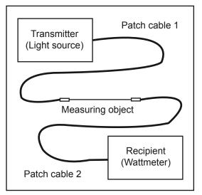
Unavoidable losses appear at all removable plug connections of optical fiber cables due to their functional principle. These losses are determined by the precision of the alignment of the respective fiber end surfaces and the quality of the fiber end polishing. The insertion loss is a measure for the apparent losses at these plug connections and therefore of the quality of the plug assembly (Insertion Loss, IL, see also chapter 7 Vacuum Optics).
