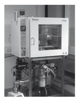
Vacuum components can be baked out to achieve a further reduction of the outgassing rate. The desorption and diffusion rates of all materials are highly temperature dependent. Therefore, the material surfaces are freed from adsorbed particles at high temperatures (e. g. 300 °C) while the diffusion of molecules in the material will be accelerated. Thus the bakeout reduces the outgassing rate during the future operation under low pressures.
