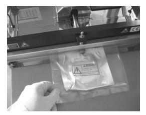
All products are packed in such a way that the cleanliness achieved during the ultrasonic cleaning process including freedom of oil and grease will be preserved. In addition, we can provide cleanroom packaging (ISO class 7).
