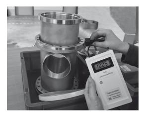
The magnetic permeability  $\mu$  characterizes the permeability or magnetic conductivity of materials. It is the product of the magnetic field strength  $\mu_0$  and the relative permeability  $\mu_r$ , which we can determine for paramagnetic materials ( $\mu_r = 1...2$ ).
