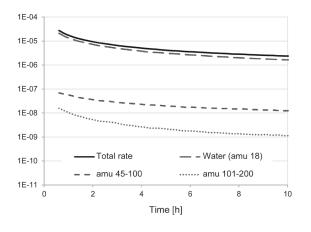
The evaluation of the outgassing behavior of materials, components and assemblies is most important for many modern technology processes. This includes on the one hand the basic classification of materials regarding their vacuum compatibility that depends both on the operating pressure and the prevailing temperatures.
