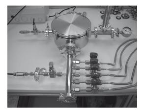
You want to know how your vacuum chamber/assembly behaves in operation and determine the outgassing behavior? We provide you with the opportunity to bakeout complete vacuum chambers and to determine the outgassing and the outgassing rate by means of mass spectrometry.
