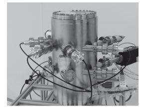
Vacuum gauges are instruments which have to be controlled regularly according to DIN EN ISO 9001-2000.
